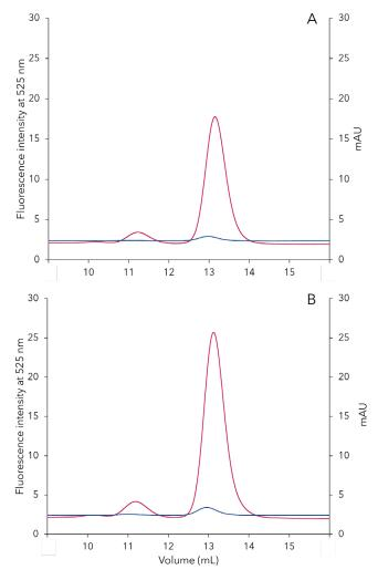
Fig. 2 Overlay of FITC-BSA peak measured with fluorescence (red) and UV 280 nm (blue). Sample 1 with 0.8  $\mu$ g (A) and sample 2 with 1.3  $\mu$ g (B).
