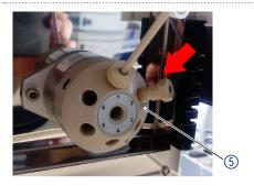
Insert the 1/16"capillary (3) into the fitting (2). Tighten the nut
