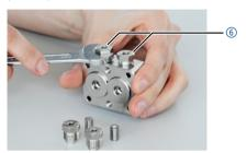
Fig. 22: Removing lower bushings
