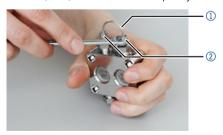
Fig. 19: Removing capillary connection
