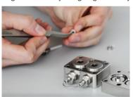
Fig. 13: Separating backing ring and adjusting ring
