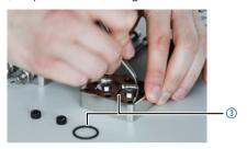
Fig. 18: Removing o-rings
