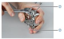
Fig. 28: Tighten bushings
