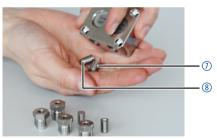
Fig. 23: Removing check valves
