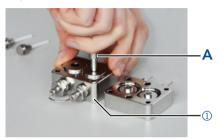
Fig. 16: Removing seals (high-pressure side)
