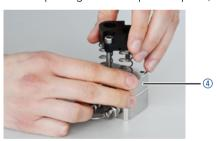
Fig. 9: Removing piston guide
