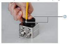
Fig. 8: Removing cylinder bolts
