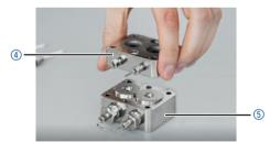
Fig. 11: Separating pressure plates
