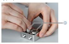
Fig. 25: Reinserting inlays
