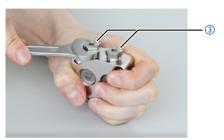
Fig. 20: Removing upper bushings
