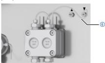
Fig. 5: Removing tubing of piston backflushing
