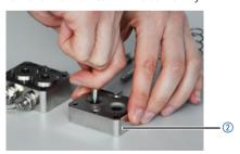
Fig. 17: Removing seals (low-pressure side)
