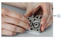
Fig. 36: Inserting o-rings
