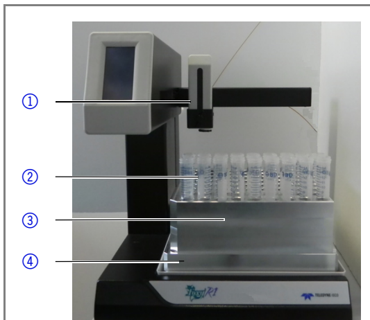
Fig. 7 Example for cooling after removing the hood
