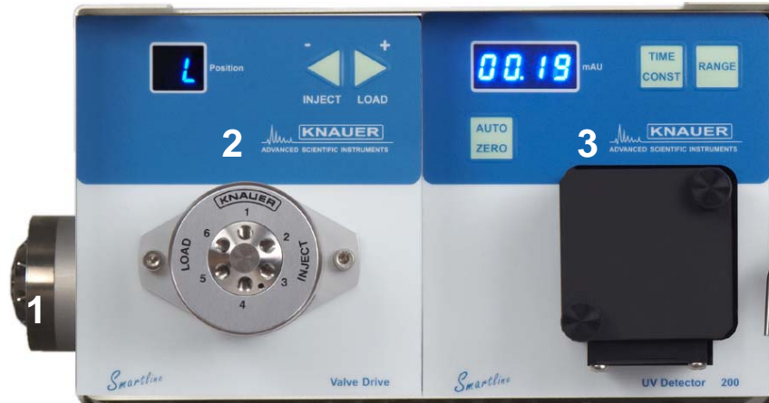
Fig. 2 Front View of the Smartline Assistant 6000 (A5003V416), including: 1 17-port/1-channel valve for fraction collection 2 6-port/2-channel valve for the injection switching 3 Fixed wavelength detector S 200 (optional)
