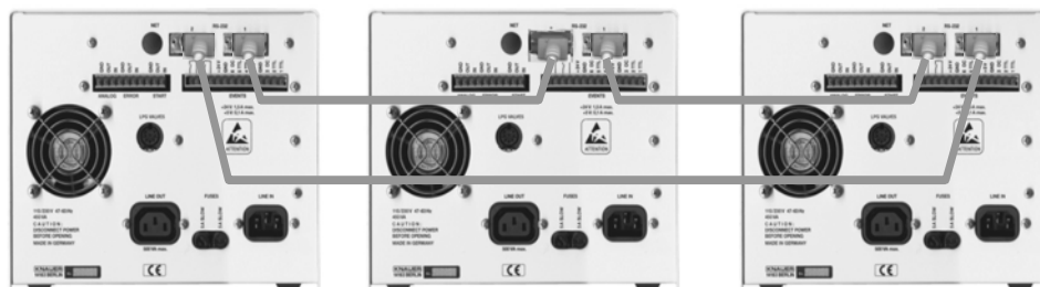
Fig. 28 Connection scheme of three Preparative Pumps 1800
