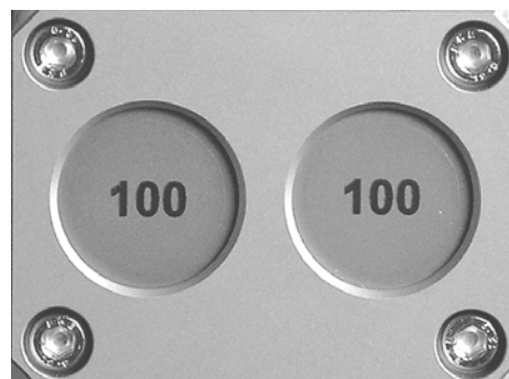
Fig. 4 Pump head identification (100ml head, inlay design)
