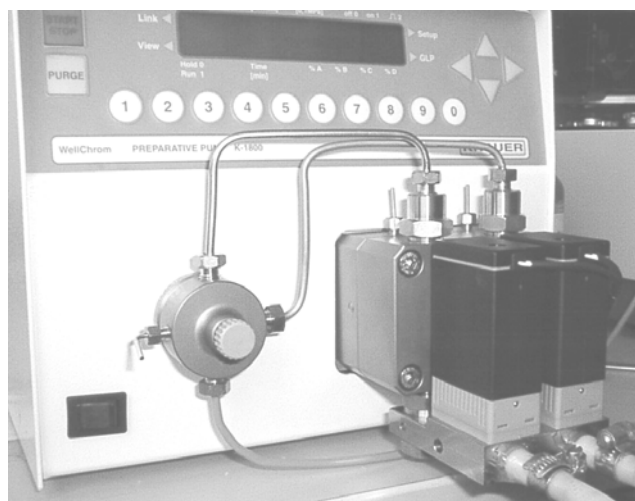
Fig. 18 Binary LPG valve block mounted to the Preparative Pump 1800
